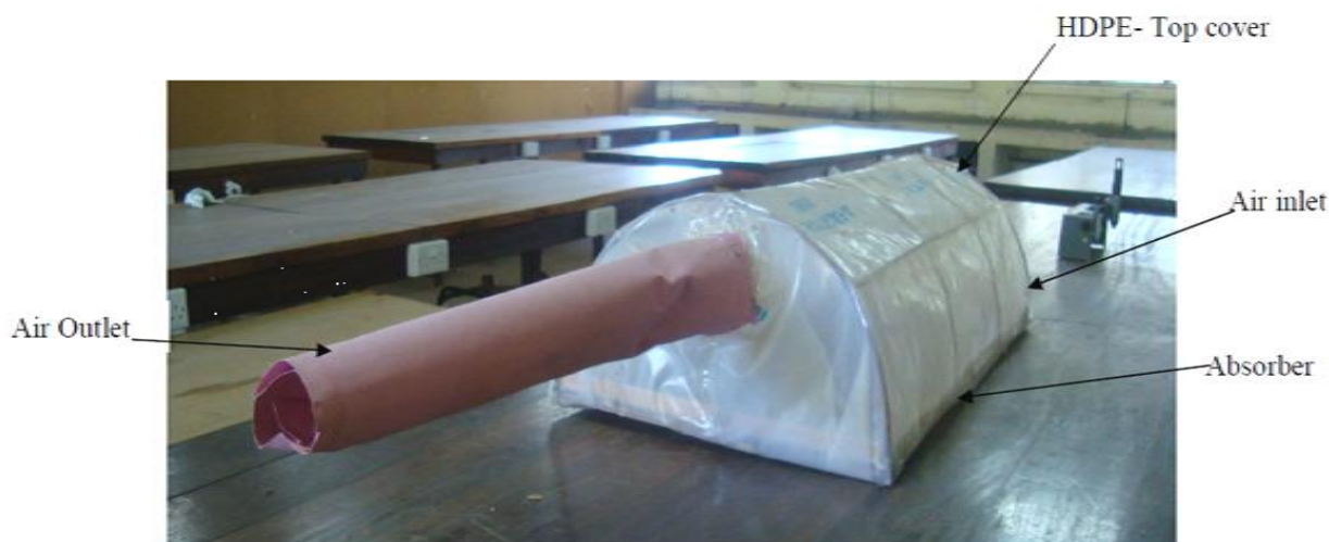
Fig. 2. The prototype of a SAH with HDPE as top cover and brown sand.
