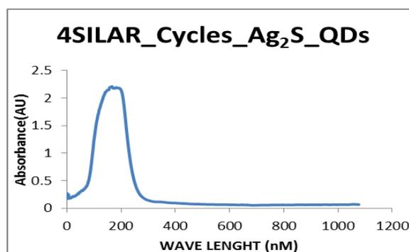
Fig. 1. UV Absorption spectra for 4 SILAR cycles of  $Ag_2S$  quantum dots with absorbance peak and wavelength.
