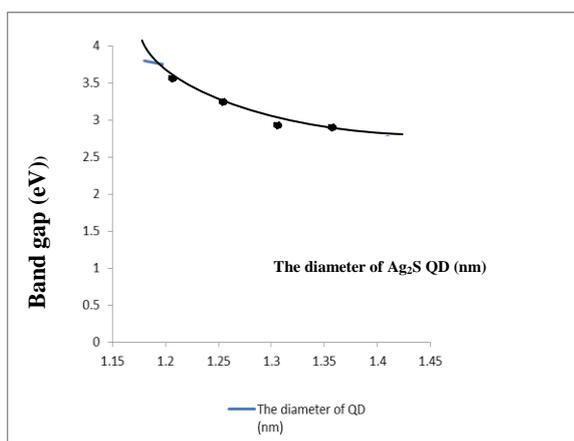
Fig. 7. A graph of band gap versus the diameter of Ag<sub>2</sub>S QDs.
