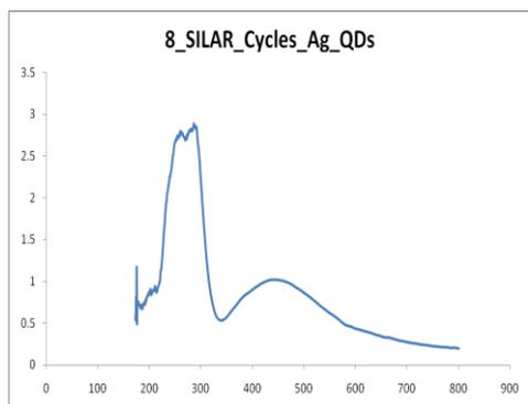
Fig. 6. UV absorption spectra for 9 SILAR cycles of Ag<sub>2</sub>S quantum dots with absorbance peak and wavelength.
