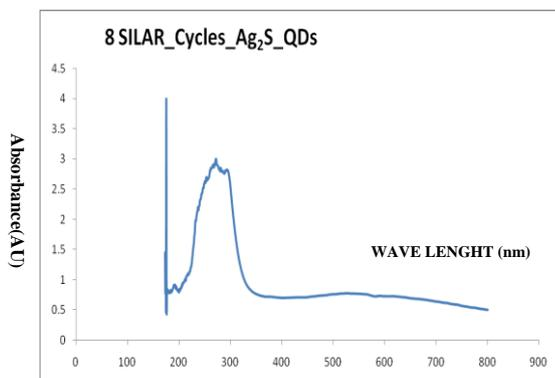
Fig. 5. UV Absorption spectra for 8 SILAR cycles of Ag<sub>2</sub>S quantum dots with absorbance peak and wavelength.
