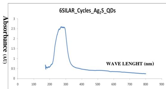
Fig. 4. UV absorption spectra for 7 SILAR cycles of Ag<sub>2</sub>S quantum dots with absorbance peak and wavelength.
