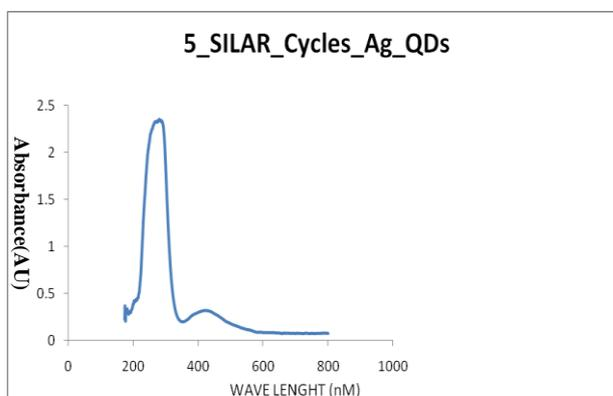
Fig. 2. UV absorption spectra for 5 SILAR cycles of  $Ag_2S$  quantum dots with absorbance peak and wavelength.
