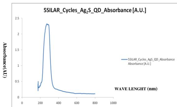
Fig. 3. UV absorption spectra for 6 SILAR cycles of Ag<sub>2</sub>S quantum dots with absorbance peak and wavelength.
