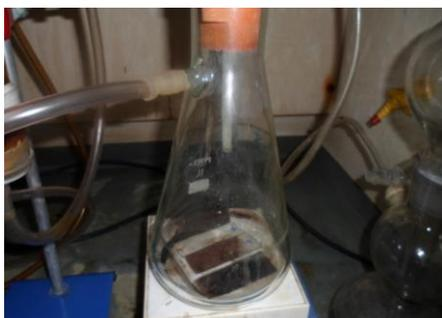
Plate 2. Sulphurization of the synthesized silver (Ag) quantum dots.
