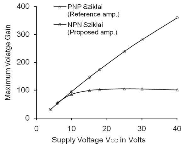
Fig. 6. Variation of maximum voltage gain with DC supply  $V_{CC}$ .
