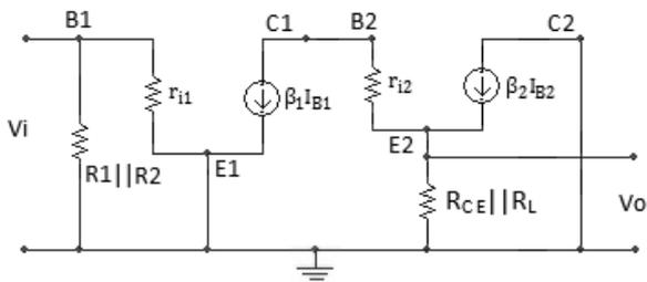
Fig. 4. AC equivalent circuit of proposed amplifier.
