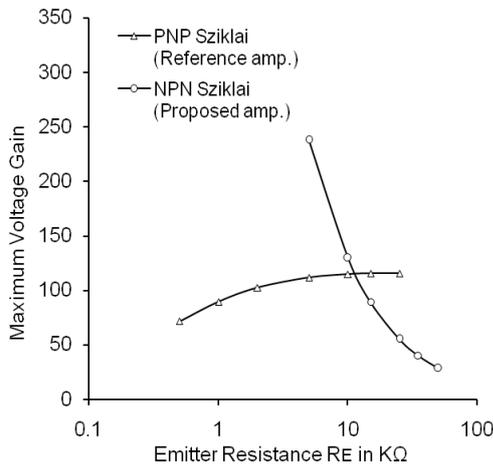
Fig. 7. Variation of maximum voltage gain with emitter resistance.
