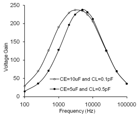
Fig. 9. Tuned frequency response of proposed amplifier at different combination of  $C_E$  and  $C_L$ .
