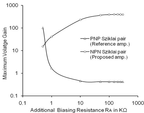
Fig. 5. Variation of maximum voltage gain with added resistance  $R_A$ .
