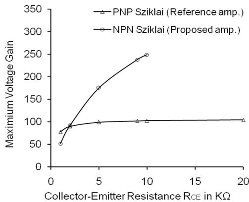
Fig. 8. Variation of maximum voltage gain with collector resistance.
