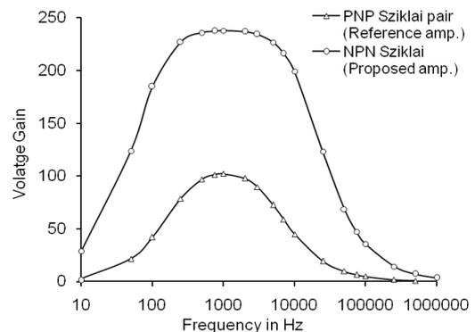
Fig. 3. Variation of Voltage gain with frequency.
