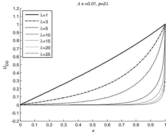
Fig. 1. The DG solution of the troesch's problem for various  $\lambda$ .
