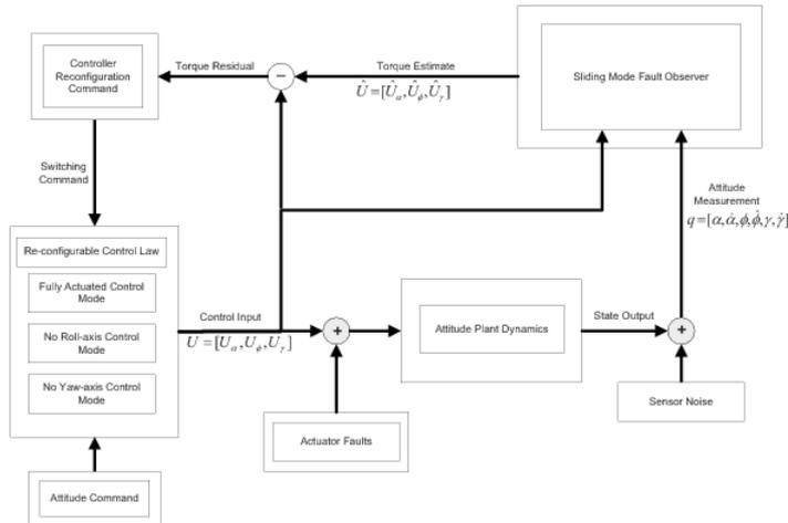
Fig. 2. Reconfigurable controller.
