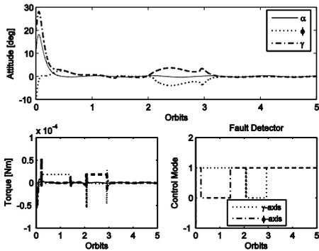
Fig. 5. External disturbance case - top: attitude states. bottom left: control effort; bottom right: fault detection logic..
