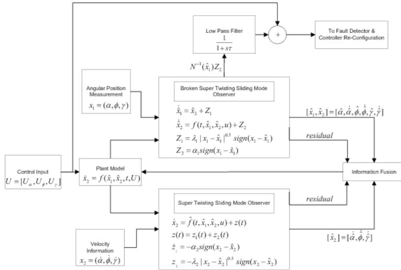
Fig. 1. Proposed sliding mode observer system for FDI.
