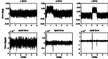
Fig. 4. External disturbance case - observer error for attitude fault recovery.
