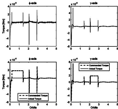
Fig. 3. External disturbance - torque estimation. Top left/right: torque estimation. Bottom left/right: commanded and actual torque.
