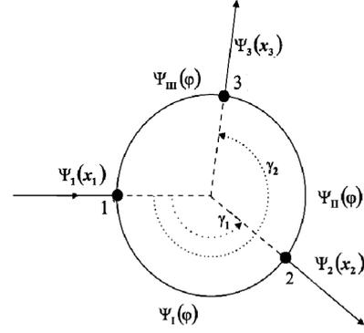
Fig. 1. The geometry of the device and the relevant wave function in the different domains. The parameter  $\varphi$  is measured from junction 1 in counterclockwise direction.
