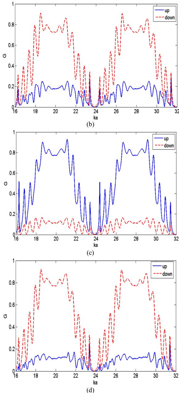
Fig. 4. (a) plot of our system, the conductance  $G/G_0$  ( $G_0 = e^2/h$ ) of ring, (b) input electrons with spin up=100%, (c) down=100% and (d) up=60% and down=40%.
