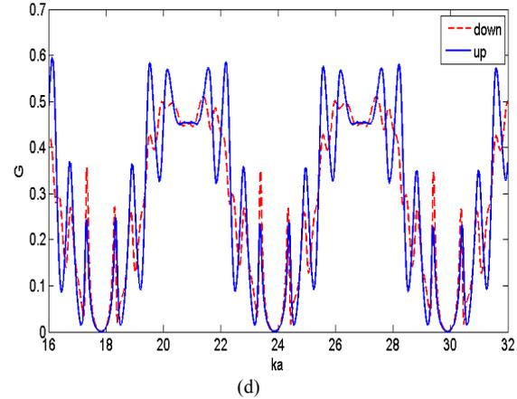
Fig. 2. (a) plot of our system, the conductance  $G/G_0 (G_0 = e^2/h)$  of ring, (b) input electrons with spin up=100%, (c) down=100% and (d) up=60% and down=40%.
